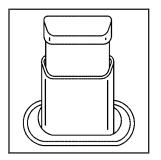
To lock the door from the inside, push the manual lock knob down. To unlock the door, pull the knob up.
